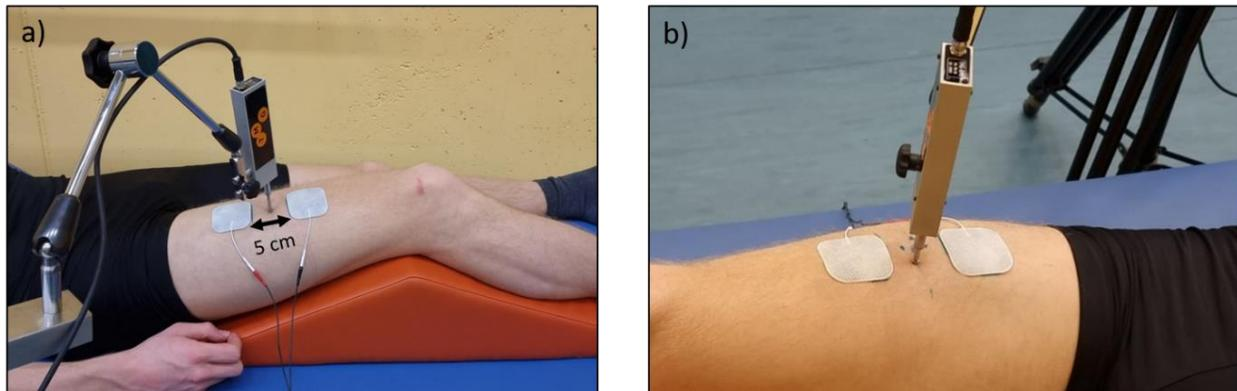
Figure 3. a) TMG measurement set-up for RF with an inter-electrode distance of 5 cm. b) Medial shift displacement of the sensor position.
