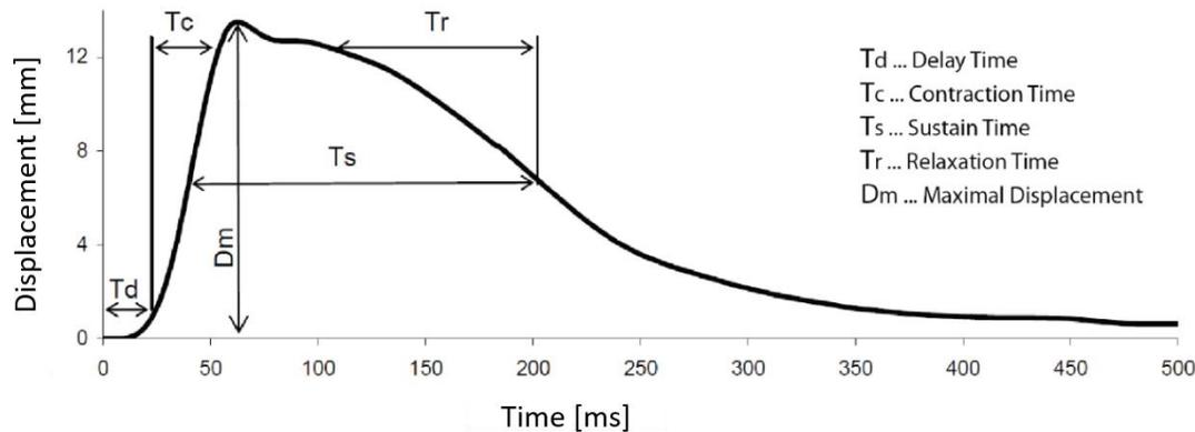
Figure 1. Exemplary displacement-time curve with the derived TMG parameters.
