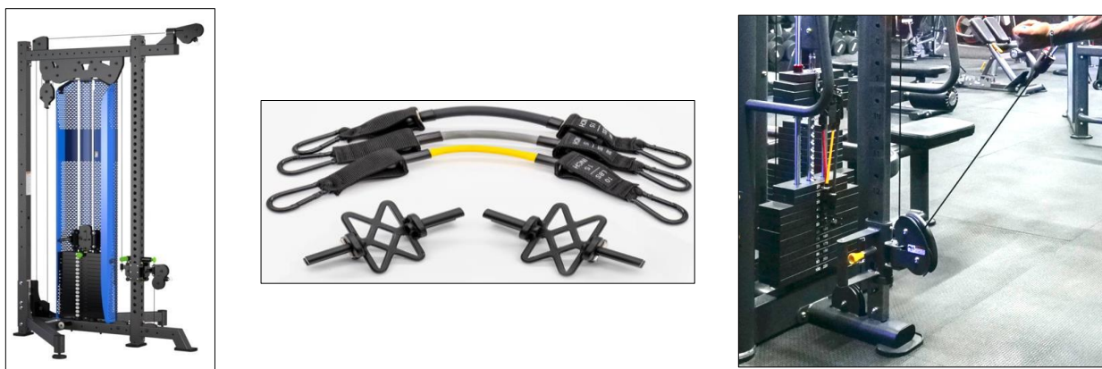
Figure 1. Selectorized resistance machine (left panel). Stack Bands ensemble (middle panel). They operate by using elastic cords pegged above and below the chosen selected weight on the machine. As a cable biceps curl is performed, the effective load on the stack (i.e., downward pull as a result of the tension in the elastic resistance bands) increases due to the tension in the elastic bands, which stretch and reach their maximum tension at the end of the concentric phase. When the arm is initially lowered (eccentric phase) the elastic cords are at their maximal resistance, providing an eccentric overload (right panel).
