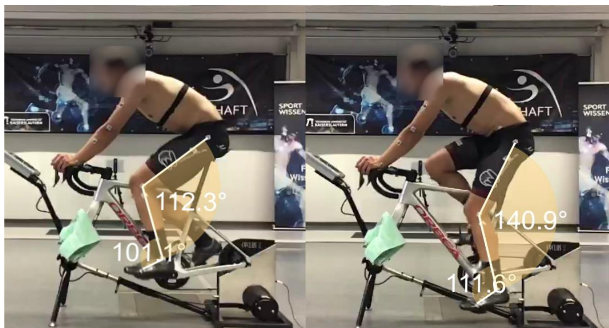
Figure 1. Measuring procedure and angle definition.
